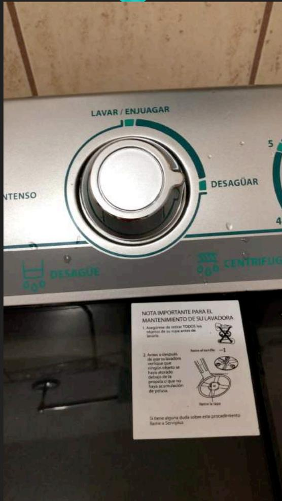
The last thing you do is move the 3<sup>rd</sup> knob from LAVAR (wash) to DESAGUAR (drain). Make sure the hose connected at the bottom is draining into the shower so excess water can run into the drain.
