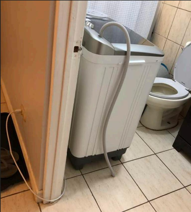
Once you have it situated, you can take the thinner hose (that can detach and hook it up to the sink-turn the sink on and the hose basically transports water into the tub of the machine
